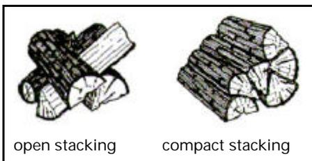
Low intensity fires cause tar and creosote to deposit in the chimney after a long period of time. Tar and creosote are highly combustible substances. Thicker layers of these substances might catch fire when the temperature in the chimney increases suddenly and steeply. Therefore it is necessary for the fire to regularly burn very intensely, so that thin layers of tar and creosote immediately disappear.
