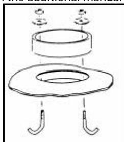
Put the heat shield back before connecting the stove to the chimney.
